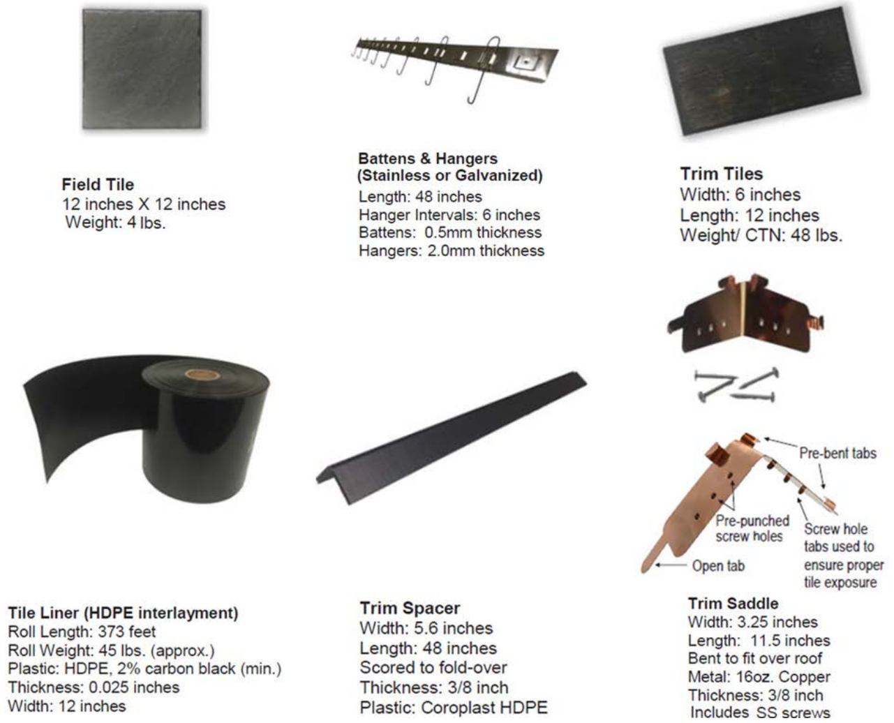
FIGURE 1—IRONSTONE ROOF COVERING SYSTEM AND ACCESSORIES
