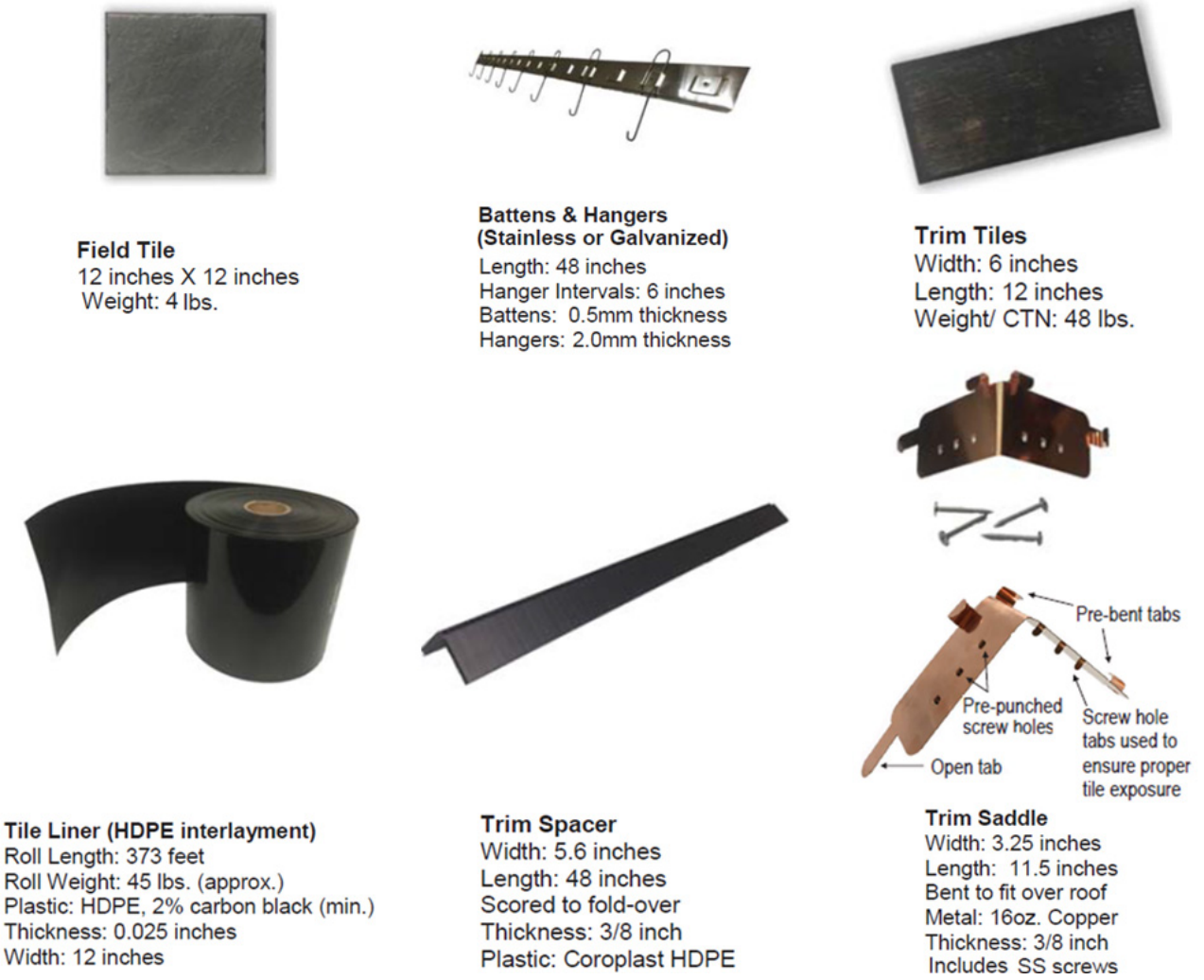
FIGURE 1—IRONSTONE ROOF COVERING SYSTEM AND ACCESSORIES
